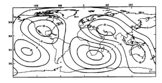
Data not corrected for ellipticity; Notice large zonal  $P_{20}$  term negative at the equator
